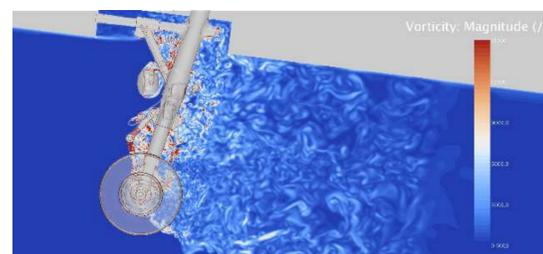
Nose and main landing gears are main contributors of airframe noise.
