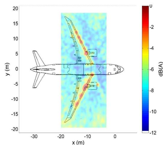
Advanced algorithms for enhance sound source localization, particularly low frequency methods, have been developed.
