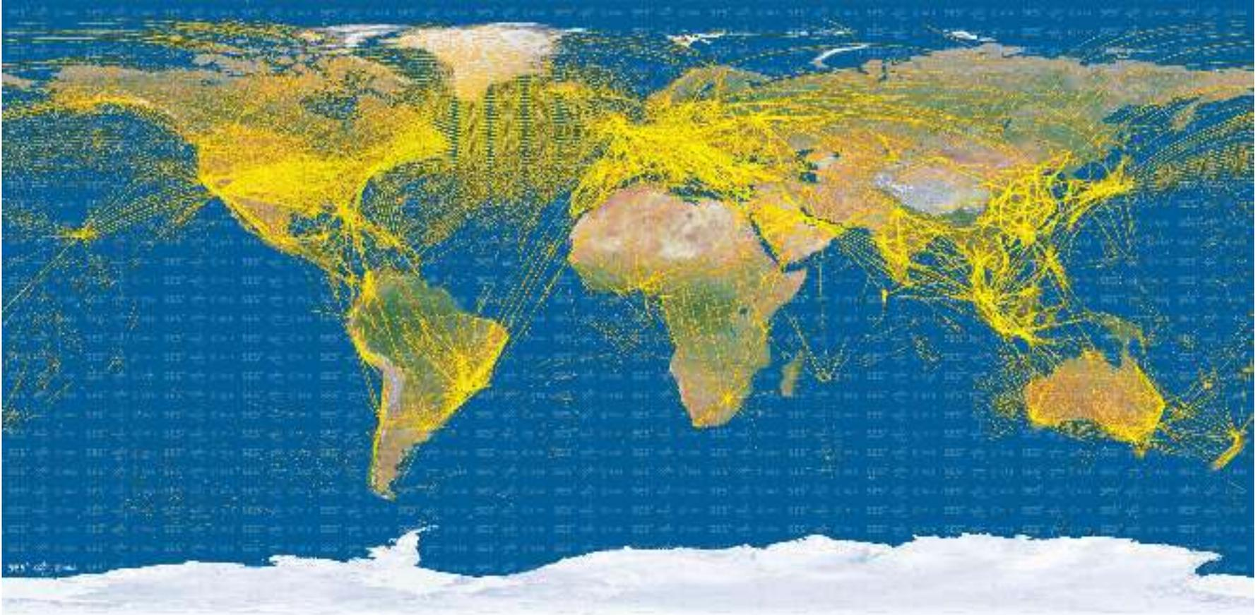
*DLR/SES experiment to detect Automatic Dependent Surveillance Broadcast (ADS-B) aircraft signals using the Proba-V microsatellite (<https://phys.org/news/2015-05-proba-v-world-air-traffic-space.html>)*
