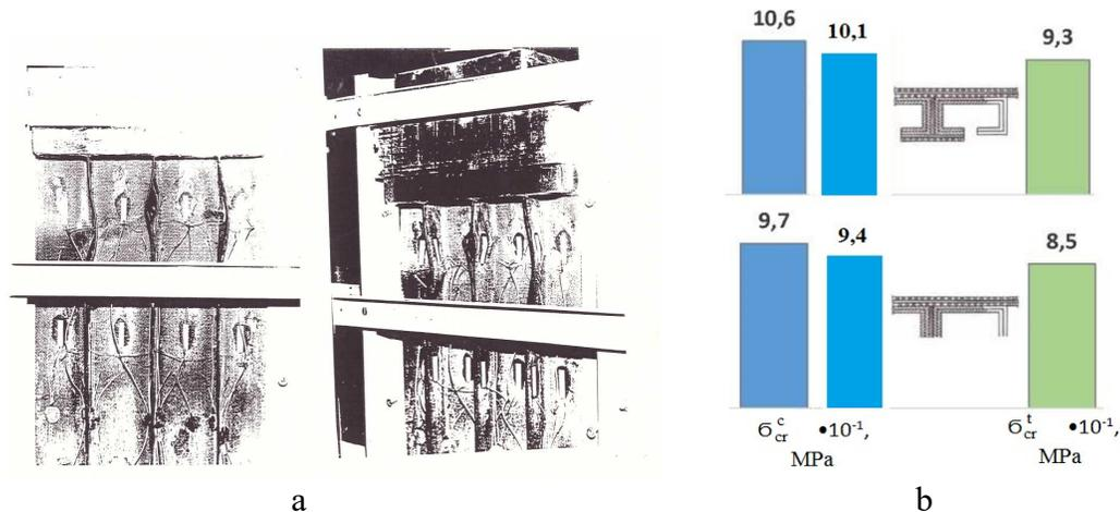
**Figure 3. Stringer panels compressed in the longitudinal direction: (a) experimental specimen; (b) comparison of the test and calculation results for critical stresses**
