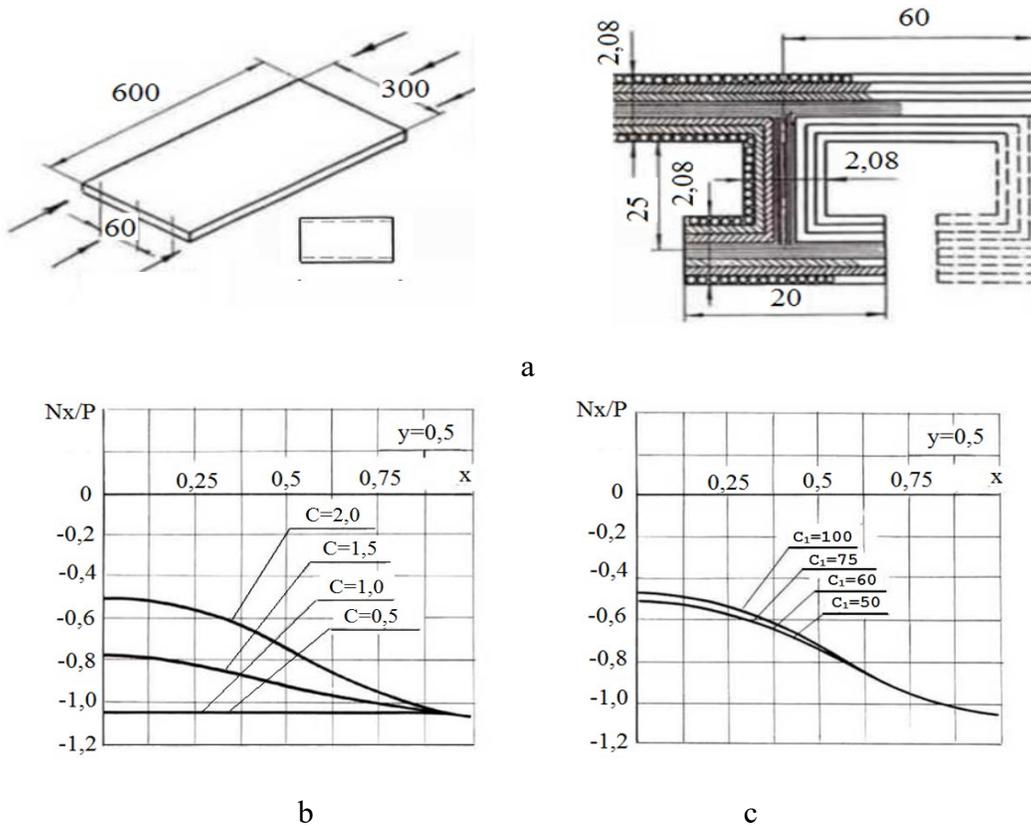
**Figure 1. Stringer panel compressed in the longitudinal direction: (a) panel sizes, layout of the package and stringer geometry; (b) dependence of normal forces on panel side ratio under in-plane bending; (c) dependence of normal forces on stringer distance under in-plane bending**
