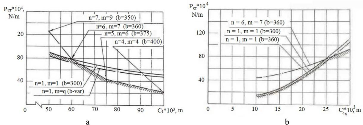
**Figure 2. Stringer panel compressed in the longitudinal direction: dependence of critical forces of bending mode and torsion mode of buckling (a) on stringer distance; (b) on height of stringer cross section wall**
