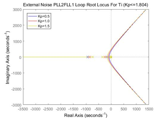
**Fig. 15** equivalent root locus cluster for pi compensation of the system
