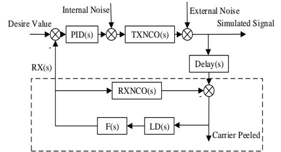
**Fig. 11** carrier self-alignment loop block diagram with PID compensation
