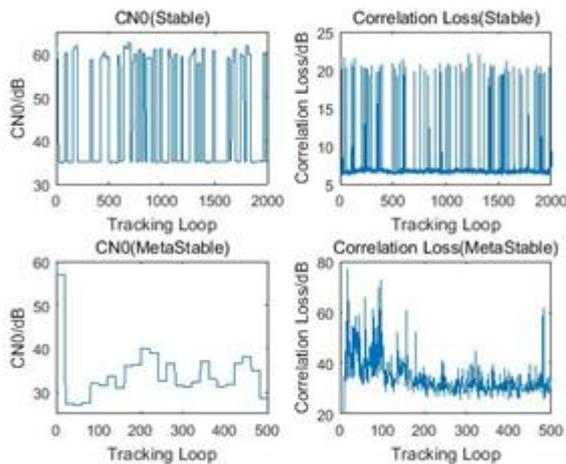
Fig. 1 carrier noise ratio in the stable and metastable state
