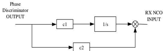
Fig. 7 second order loop filter block diagram
