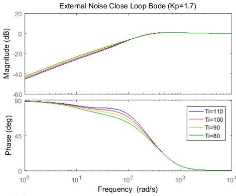
**Fig. 16** bode diagram of different integral time constants in the system
