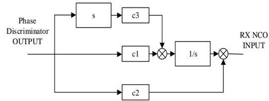
Fig. 8 second pll loop filter assisted with first flf block diagram
