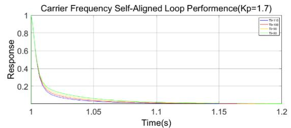
**Fig. 19** performance of different integral time constants for the unit step signal input response
