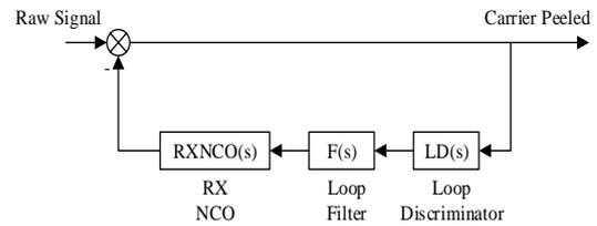
Fig. 9 receiver carrier loop block diagram
