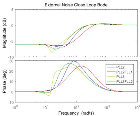
**Fig. 14** system bode diagram for external noise input
