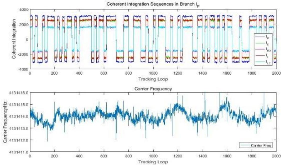
**Fig. 1** coherent integration and carrier frequency in the stable state
