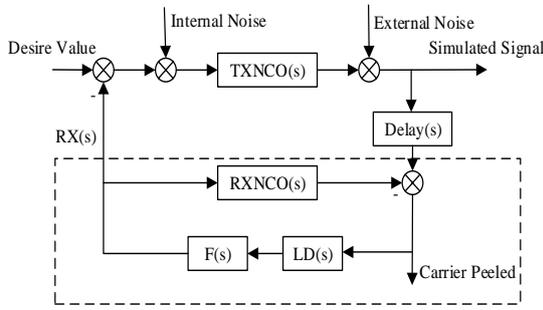
**Fig. 10** pseudolite carrier frequency self-alignment closed-loop system block diagram
