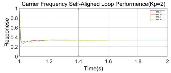
**Fig. 17** the unit step response of different loop filters in the system
