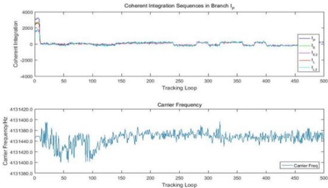
**Fig. 2** coherent integration and carrier frequency in the metastable state
