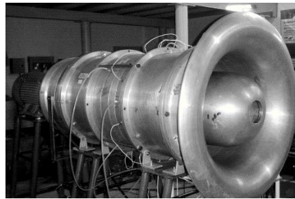
Fig. 5 Low-speed three- stage compressor test rig (Nie et al. [7]).
