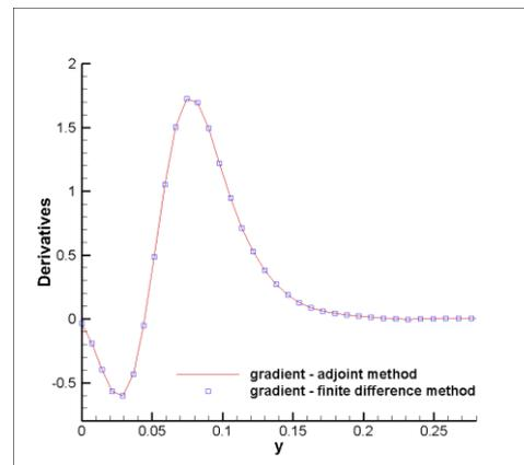
**Fig. 3** Verification of adjoint method with the comparison of finite difference method
