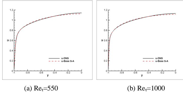
**Fig. 2** Comparison of u profile between DNS and S-A turbulence model
