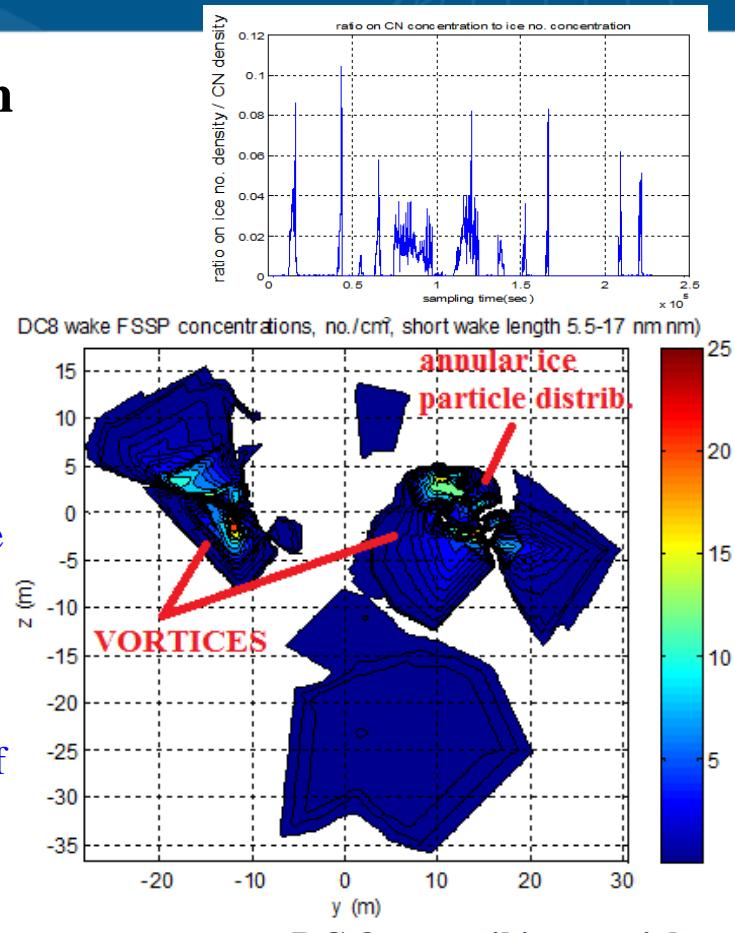
DC-8 contrail ice particle distribution dominated by TWV, trailing wake vortex pair of vortices
