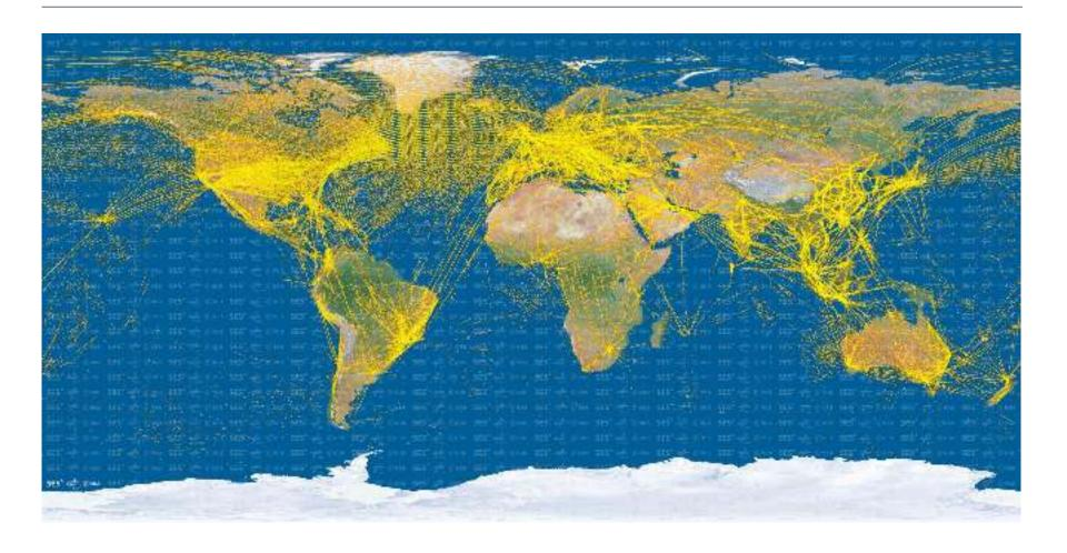
DLR/SES experiment to detect Automatic Dependent Surveillance Broadcast (ADS-B) aircraft signals using the Prova-V microsatellite (https://phys.org/news/2015-05-proba-v-world-air-traffic-space.html)
