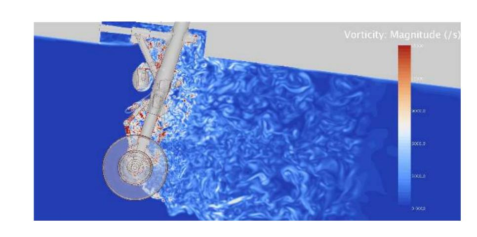
Nose and main landing gears are main contributors of airframe noise.
